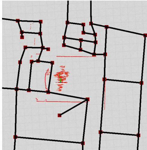
Figure 2: Demonstration of the auto-complete graph (ACG). The prior map (in this case extracted from a crude line drawing) is shown with black lines (corners as brown squares). The current live sensor data (2D lidar) is shown with red points. The particle cloud, used in an MCL implementation that localises the sensor data against the prior map, is shown as red arrows.
